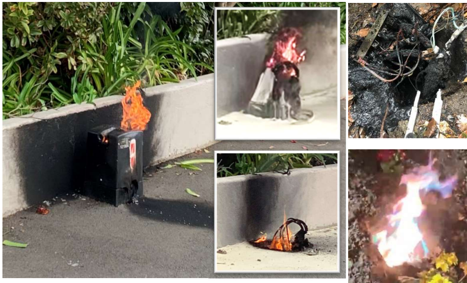
Figure 1 – Example of a plastic pillar on fire at different stage, from start to end (left) and two other pillars on fire and the remains after fire (Reproduced from [6])
